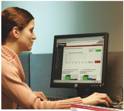
With just a few mouse clicks, management can view OEE calculations by work-cell, downtime/machine, quality data, changeover times and the causes of stoppages.
