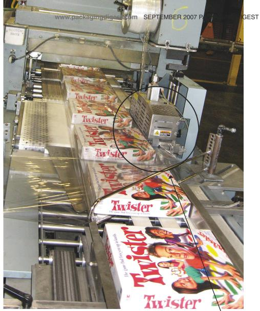
In 2005, Hasbro installed hot-knife side sealers (arrow) on its case packers. The sealers produce a narrow seam (below) that does not block the graphics on the sides of the boxes.
