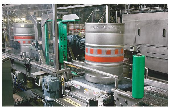
The in-motion checkweigher with control panel, above, weighs half-barrel kegs (160 lb) and can also be quickly changed over to run quarter barrels.
