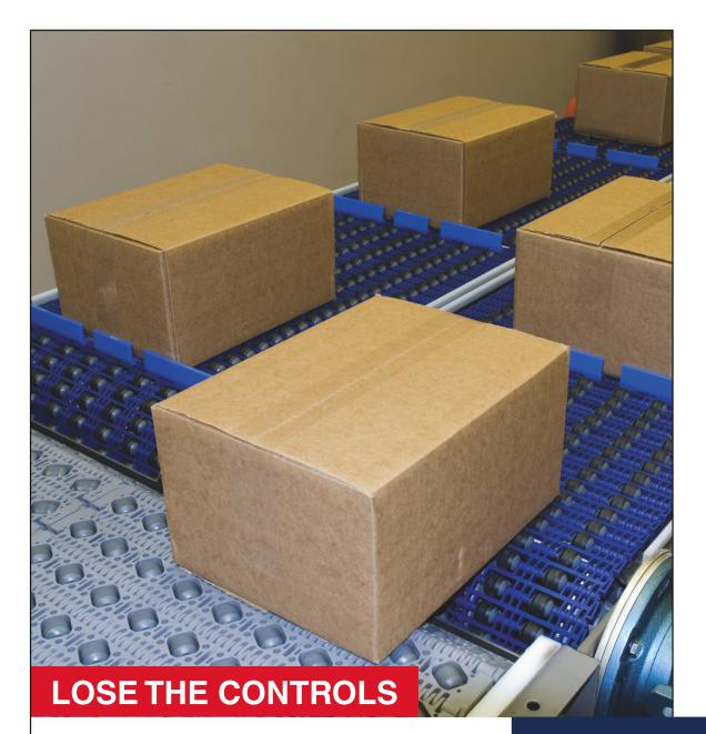
Intralox's perpetual merge system realizes a steady-state product flow of two or more conveyor lines into one without using accumulation or controls. The patented technology of this compact merge solution automatically staggers products before entering a merge without the stops and starts
