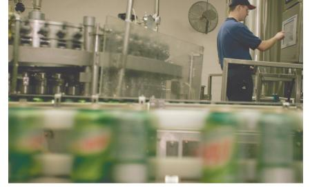
Sanitized cans reach the filler room and make their way through a 72-valve filler station, which operates at speeds of up to 1,200 cans/min.
