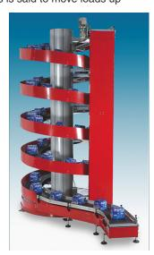
load capacity is 75 lb/linear ft for speeds to 200 ft/ min, with angle of incline between 9 and 11 deg to safeguard against loads sliding or tumbling. Friction inserts are available for slick products/packages.
