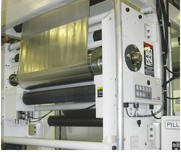
The mid-web press, above, can tackle multiple substrates, including unsupported film, paper and carton board. The press's overhead web path, left, allows operators safe access to the printing and laminating modules.
