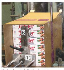
Hasbro has installed horizontal case packers to run the wide range of box sizes required for the many games it runs in its plant.
