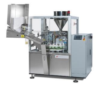
Tube filler The 602 is introduced as the co.'s extremely compact tube-filling machine, one that fills and seals at rates to 60/min. Claimed for the machine are quick changeovers, optimum accessibility, a Mitsubishi PLC with a touchscreen, seven levels of password-protected security, up to 30 pre-programmed format tables and a modem for remote access and the downloading of production statistics.
