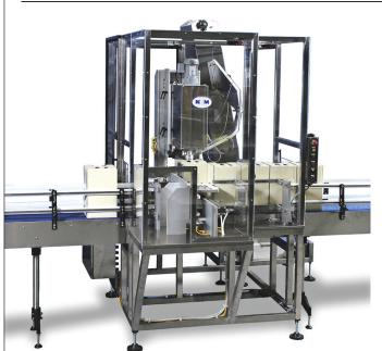
Capper The NESHC bows in as a continuous-motion, single-head capper for large containers, and is designed to handle various closure finishes and container varieties. The co. cites the freestanding machine's highly accurate indexing turret which provides positive chuck-cap application to ensure straight and secure closures. An adjustable feature handles singles and twin-packs.
