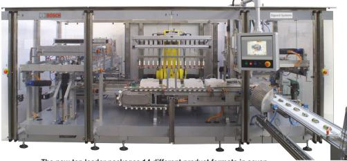
The new top loader packages 14 different product formats in seven different tray sizes. All supply lines for vacuum, pneumatic and electrical sensors are integrated in a connecting plate, which holds the product gripper. This makes it very easy to change the gripper for a new product format, as the operator does not have to worry about the reconnection of additional cables and plugs.
